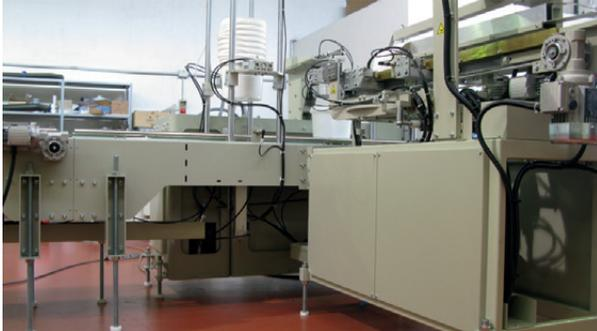
The machine is provided with a close-packed loading system for handles for manual loading; the handles are loaded one by one and the ratio between loading/consumption is 5:1;
